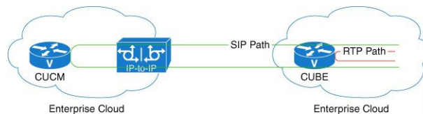
Figure 16: Anti-Tromboning - Avoiding Media Loops
