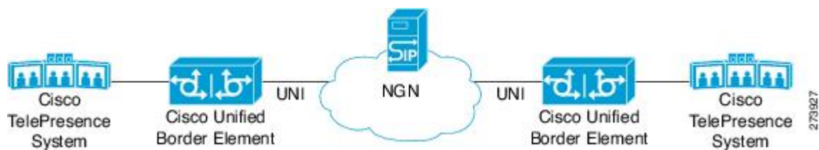
Figure 26: Cisco NGN with CCUBE providing UNI interface
