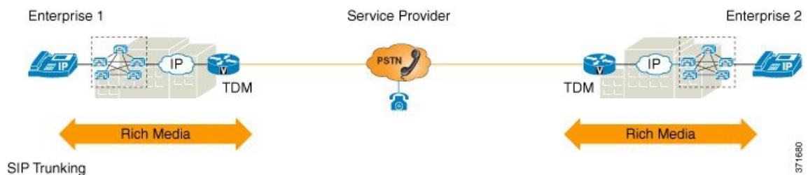
Figure 4: SIP Trunking Overcomes TDM Barriers
