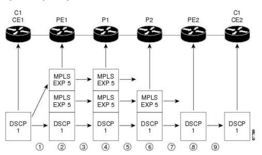
Short Pipe mode functions as follows. The circled numbers at the bottom of the illustration correspond to the step numbers.
