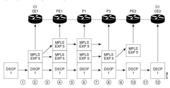
Pipe mode with an explicit NULL LSP functions as follows. The circled numbers at the bottom of the illustration correspond to the step numbers.
