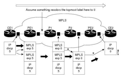
\*In both the MPLS-to-MPLS and the MPLS-to-IP cases, the PHBs of the topmost popped label is copied into the new top label or the IP DSCP if no label remains
