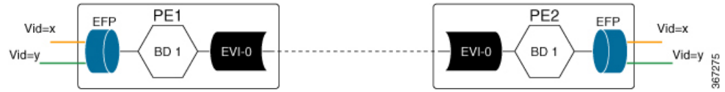
Figure 48: VLAN Bundle Service Interface
