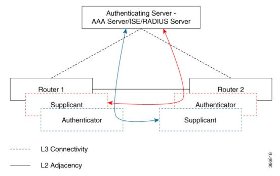
When the interface is configured for 802.1x role as both, The authentication manager on a router creates a session with two EAP session (blue and red with separate EAP session ID) flows with supplicant as well as an authenticator role and both trigger EAP-TLS mutual authentication with the remote authenticating server (AAA server/ISE/RADIUS).
