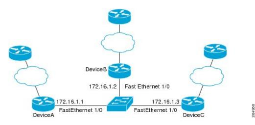
The example, starting in global configuration mode, shows the configuration of BFD.
