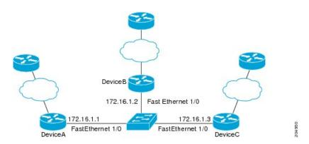
When Fast Ethernet interface 1/0 on RouterB fails, BFD will no longer detect Router B as a BFD neighbor for RouterA or for RouterC. In this example, Fast Ethernet interface 1/0 has been administratively shut down on RouterB.
