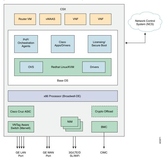
Figure 4-1 vWAAS as VNF in Cisco Enterprise NFV
