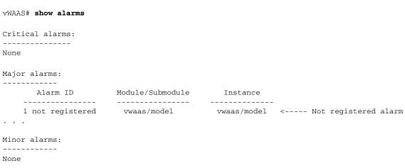
Figure 8-1 Display for show alarms Command: Not Registered Alarm
