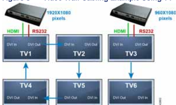
Figure 8 Video Wall Cabling Example Using TV Tile Matrix Functionality
