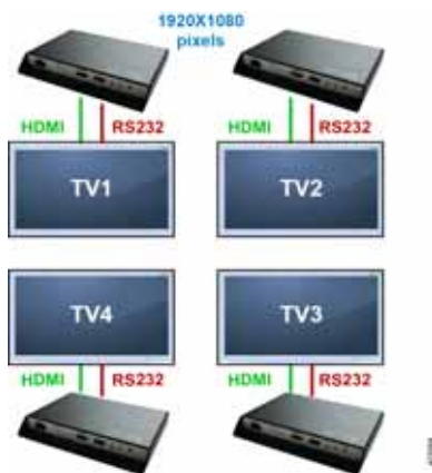
Figure 1 Cabling Video Wall with One DMP Per TV Display
