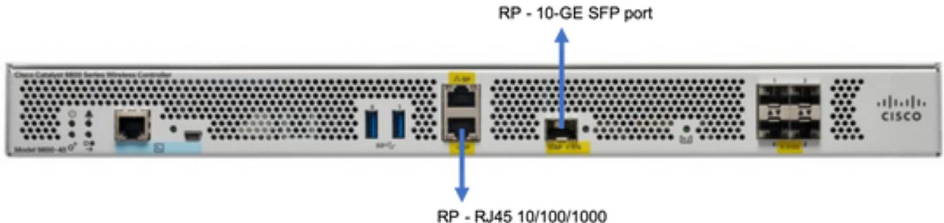
**Note:** In Cisco IOS XE 16.10 to 16.12, it is recommended to connect the 9800s Redundancy Port to the same switch where the management connection of the 9800 is connected (see network topology). This is because there is no verification for the gateway reachability in these versions. A back-to-back connection works but cause higher chances of 9800 controllers to become active-active when connected that way. Note that the RP port does not use vlan tagging.
