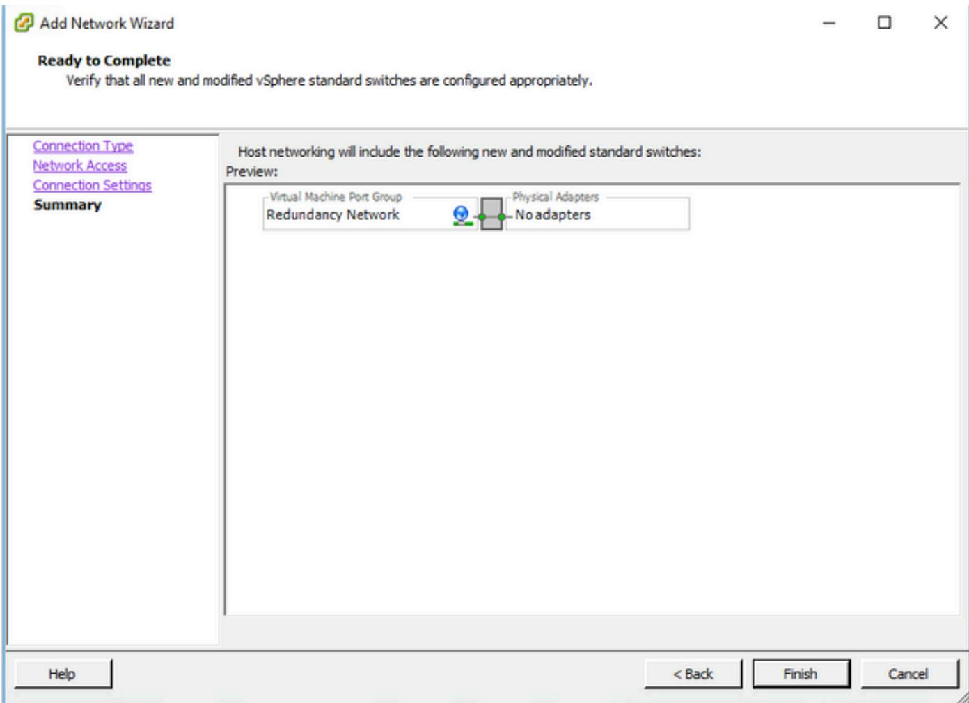
Step 6. Link an interface from both virtual 9800 WLCs (one of every virtual 9800 WLC) to the Redundancy Network.
