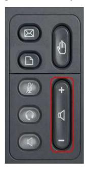
Using the volume adjuster, scroll up and down to adjust the ringer volume to the desired volume.
