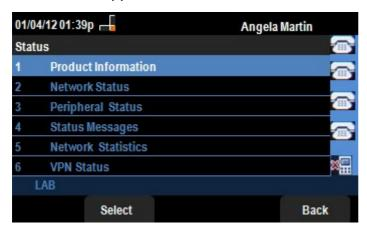
Step 3. Use the navigation keys and scroll down to VPN Status. Press the **Select** softkey. The *VPN Status* menu appears.
