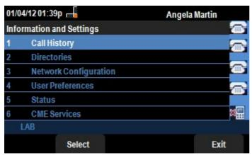
Step 2. Use the navigation keys and scroll down to Status. Press the **Select** softkey. The *Status* menu appears.
