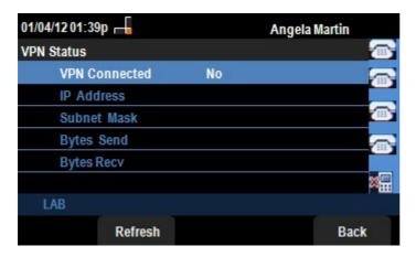
Step 4. The **Refresh** softkey can be pressed to reset the VPN connection. To go back to the previous Status menu press the **Back** softkey.
