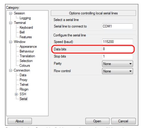
Step 8. In the *Stop bits* field, enter the number of bits to be sent at the end of every character. The stop bit informs the machine that it has reached the end of a byte. The recommended value is **1**.
