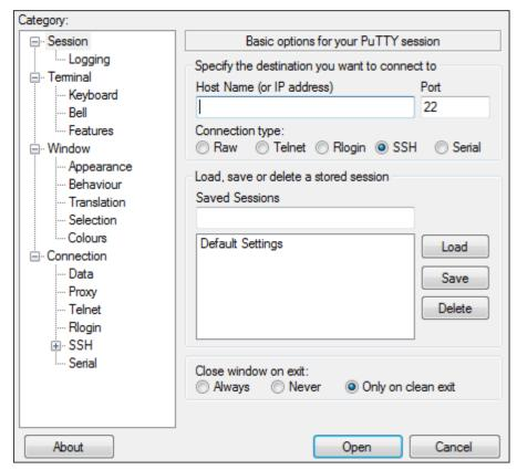
Step 3. Under the *Connection Type* field, click the **Serial** radio button.
