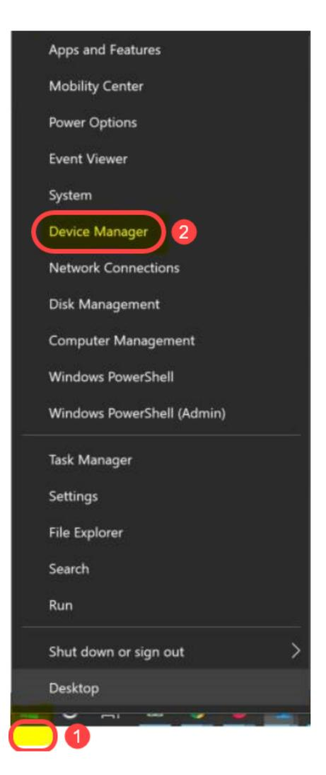
In the Device Manager, you would look to see what COM port is given to the USB adapter. In this case you would need to use COM4 for the Serial line to make the connection.
