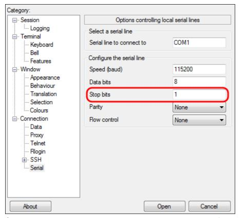
Step 9. In the *Parity* drop-down menu, select the method of detecting errors in transmission. The recommended method for detecting errors in transmission is **None**.
