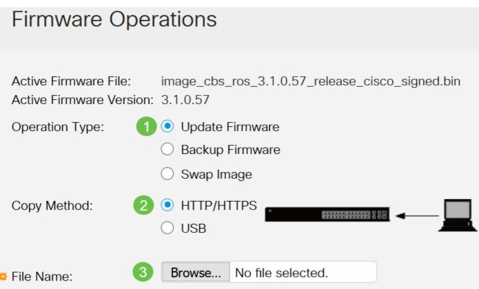
The transfer method options will vary based on your switch model. For CBS250/CBS350 series you can choose **USB** if you would like to transfer firmware to the switch using a USB flash drive. In CBS220 series switches, TFTP transfer method is available.
