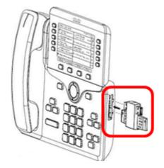
Step 5. Connect the other end of the spine connector to the KEM.
