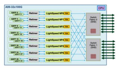
The next few sections attempt to depict the packet path to every NP. This is necessary in order to understand the punt fabric data path error message, and also in order to locate the failure point.
