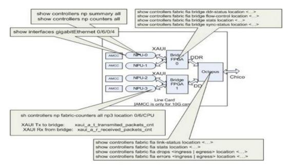
This pictorial representation helps to map each show command to the location in the data path. Use these show commands in order to isolate packet drops and faults.
