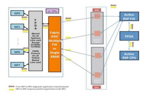
Packet Path Between the Standby Route Processor Card and the Line Card
