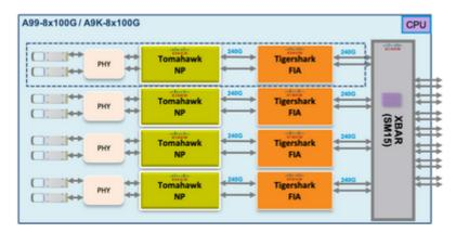
On Lightspeed and LightspeedPlus line cards the FIA is integrated in the NP chip.
