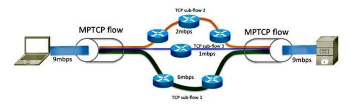
The data that enters the MPTCP connection acts exactly as it does through a regular TCP connection; the transmitted data has guaranteed an in-order delivery. Since MPTCP adjusts the network stack and operates within the transport layer, it is used transparently by the application.
