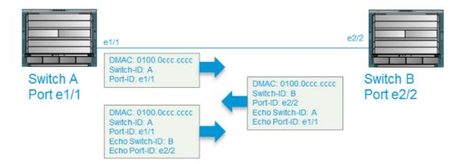
The UDLD error conditions exist when the switch does not receive the expected information from its UDLD peer.
