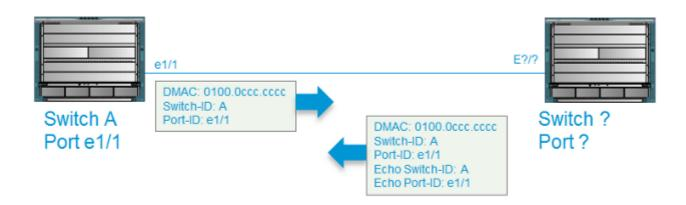
When a Tx-Rx loop is detected, UDLD performs these actions:
