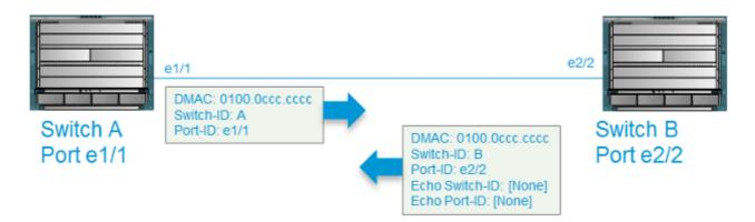
When an empty-echo is detected, the UDLD performs these actions:
