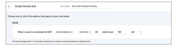
**Figure 5.** Configure density rules for specific locations, buildings, floors, and zones
