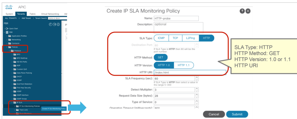
Figure 131. IP SLA monitoring policies (HTTP)
