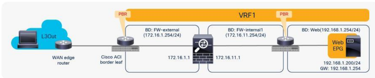
Figure 32. Intra-VRF design (L3Out EPG to Web EPG)
