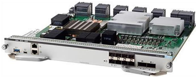
Figure 5. C9400-SUP-1 supervisor engine
