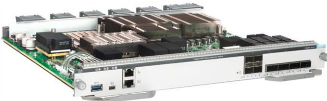
Figure 2. C9400X-SUP-2 supervisor engine
