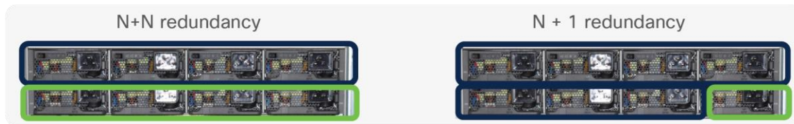
Figure 10. Power redundancy modes
