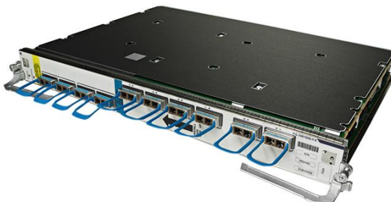
Figure 2. 10-Port 100-Gbps LSR Line Card with Cisco AnyPort Technology and Cisco CPAK Optics
