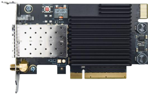
Figure 1. Cisco Nexus K35-S FPGA SmartNIC
