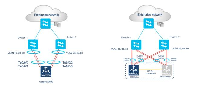
Note: Controller with multiple LAGs can be connected to a single switch, However, different VLANs must be connected to different LAGs
