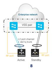
Connecting a C9800 wireless controller HA pair to upstream switches with Release 17.1 and above
