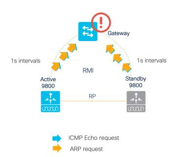
The Catalyst 9800 Wireless controller has two recovery states to prevent an active-active scenario.
