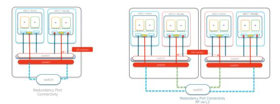
The figure on the left shows Redundant port connected on the same server.
