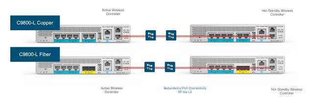
Physical Connectivity for C9800-L, C9800-40 and C9800-80 Wireless Controller HA SSO
