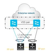
Single L2 port-channel on each box and enable dot1q to carry multiple VLANs. Spread the uplinks of the HA pair across the VSS pair and connect the RP back to back (no L2 network in between). Make sure that switch can scale in terms of ARP and MAC table entries.
