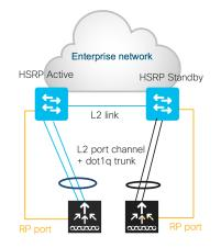
With this topology a single L2 port-channel is created on each box. Enable dot1q to carry multiple VLANs and connect the standby in the same manner. Make sure that switch can scale in terms of ARP and MAC table entries.
