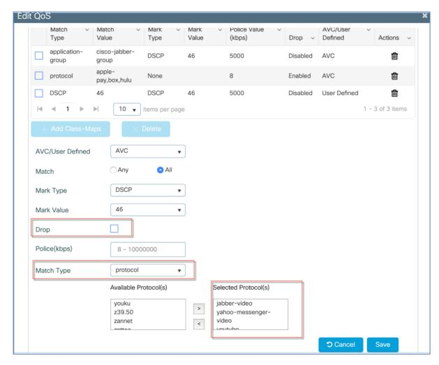
Next, select the WLAN profiles on which you want to apply this QoS policy. In the example below, we select two WLAN profiles we configured in the previous steps and applied the Ingress.
