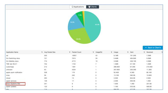
Step 3: To control the applications (Mark, Drop or Rate limit) or the traffic - configure AVC with a QoS policy to Mark/Drop or Rate Limit an application. the YouTube application.
