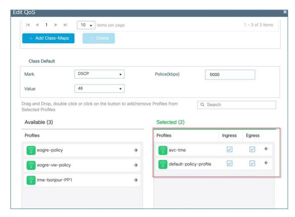
Step 4 ( Verification): Connect a client to one of the WLAN profiles configured above and try accessing different sites e.g. cisco.com and also try accessing YouTube and Twitter. The client should be able to browse to all sites except YouTube and Twitter, which are marked as dropped in the Configured QoS-policy.
