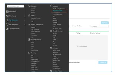
Select Configured WLANs and apply AV on them as shown in the example below, you may also select here local or external Netflow Collector
