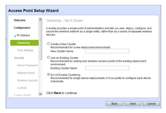
STEP 4 To create a new Single Point Setup of WAP devices, select Create a New Cluster and specify a New Cluster Name. When you configure your devices with the same cluster name and enable Single Point Setup mode on other WAP devices, they automatically join the group.
