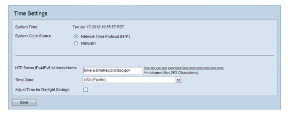
The current system time appears at the top of the page, along with the System Clock Source option.
