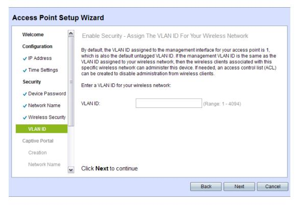
STEP 14 Enter a VLAN ID for traffic received on the wireless network.
