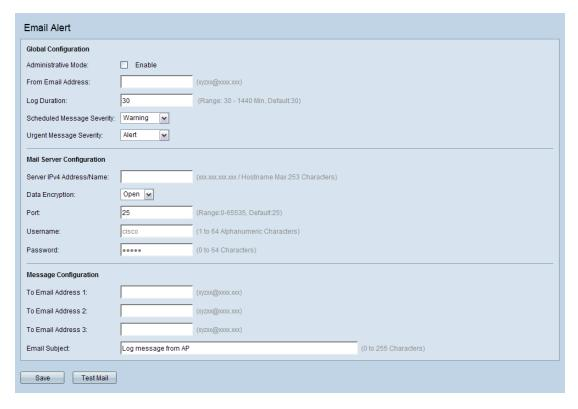
STEP 2 In the Global Configuration area, configure these parameters:
