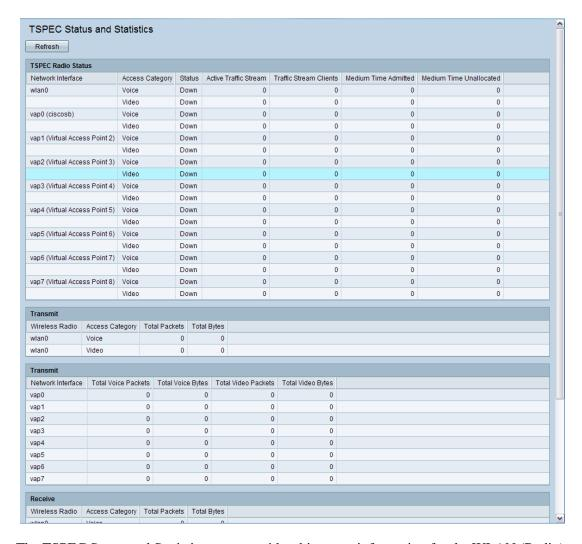
The TSPEC Status and Statistics page provides this status information for the WLAN (Radio) and VAP interfaces:
