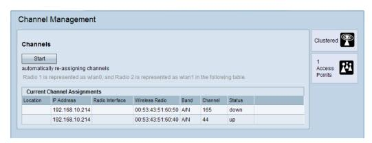
From the Channel Management page, you can view channel assignments for all WAP devices in the cluster and stop or start automatic channel management. You can also use the advanced settings to modify the interference reduction potential that triggers channel reassignment, change the schedule for automatic updates, and reconfigure the channel set used for assignments.
