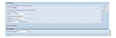
Single Point Setup is disabled by default on the WAP device. When disabled, the Enable Single Point Setup button is visible. If Single Point Setup is enabled, the Disable Single Point Setup button is visible. You can edit Single Point Setup options only when Single Point Setup is disabled.
