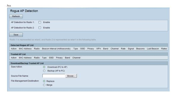
When AP detection is enabled, the radio periodically switches from its operating channel to scan other channels within the same band.
