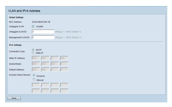
The page shows Global Settings and IPv4 Settings. The Global Settings area shows the MAC address of the LAN interface port. This field is read-only.
