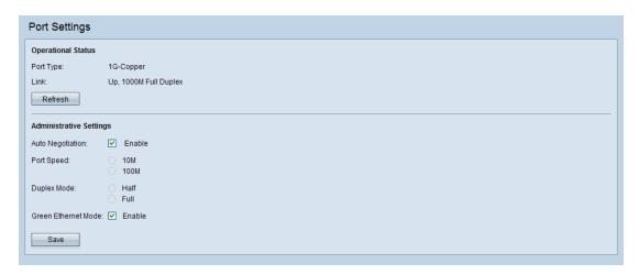
The Operational Status area shows the type of port used for the LAN port and the Link characteristics, as configured in the Administrative Settings area. If the settings change through configuration or auto negotiation, you can click Refresh to show the latest settings.
