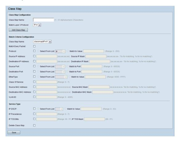
Use the fields in the Match Criteria Configuration area to match packets to a class. Select the check box for each field to be used as a criterion for a class and enter data in the related field. You can have multiple match criteria in a class.
