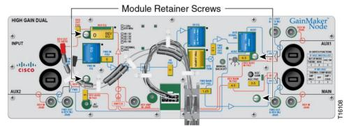
**4** Remove the RF amplifier module from the housing.
