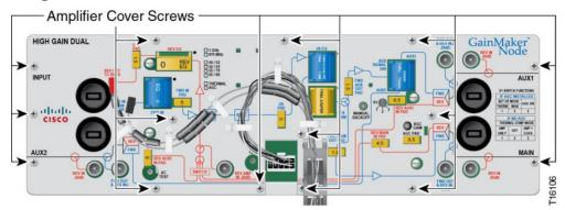
**2** Remove the RF interface board and three (3) Diplex filters using the plastic handle on the component.
