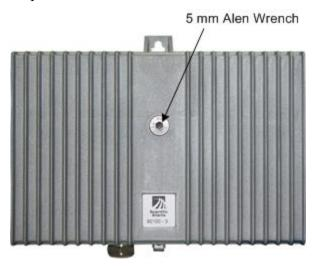
Bolt Tightening position of the node type 90100
