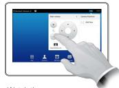
Watch the screen of your video system while using the camera controls to adjust the camera's pan tilt and zoom, if needed.
