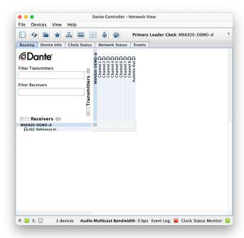
Double click the microphone's name to access its settings. First enable AES67 under the "AES67 Config" tab.
