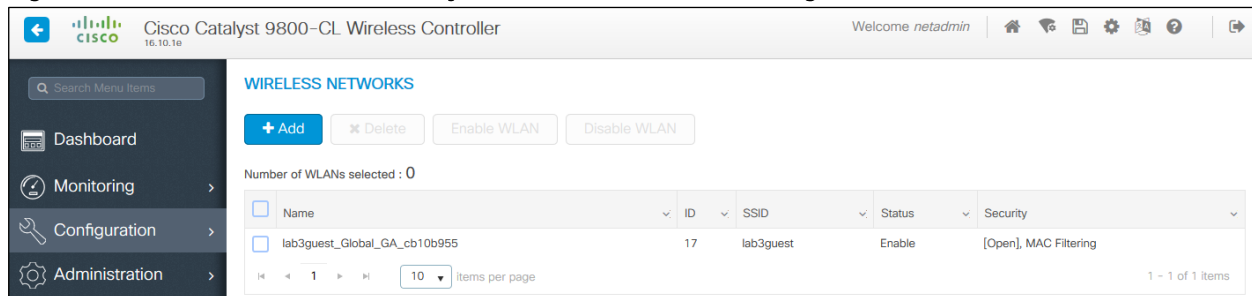
Figure 49 WLAN / SSID created by Cisco DNA Center for the guest anchor WLC
