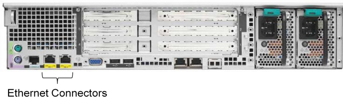
Figure 32. Cisco ADE 2140 Series Appliance Rear View
