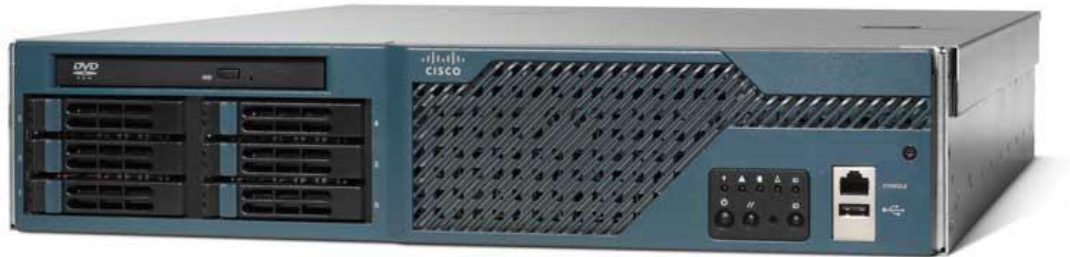
Figure 3. Cisco SV Director Server (Cisco ADE 2140) Front Panel
