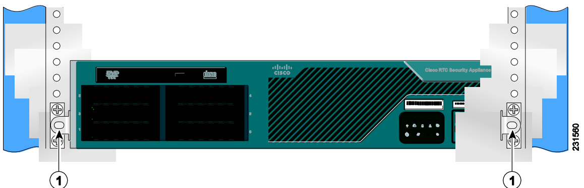
Figure 31. Securing the Appliance to the front rack posts
