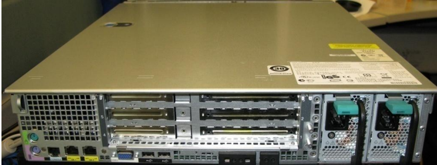
Figure 24. Cisco ADE-2140 Server – Rear View with Two AC PSUs
