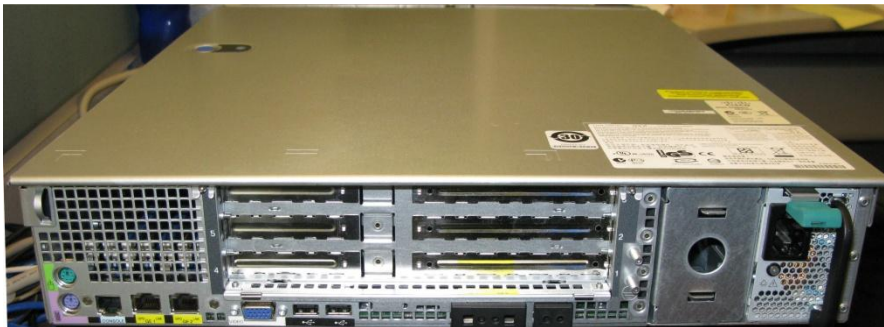
Figure 22. Cisco ADE-2140 Server – Rear View with One PSU
