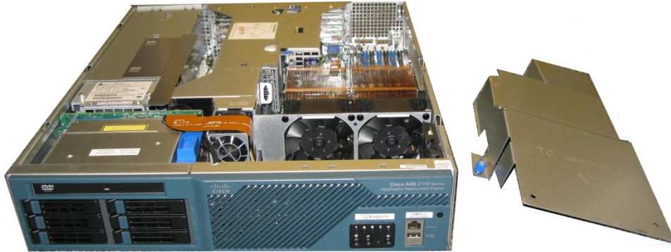
Figure 18. Cisco ADE 2140 with Air Duct Removed
