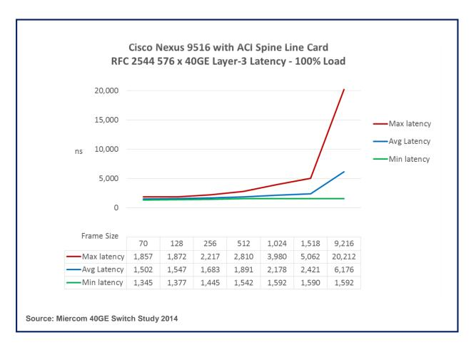
The Cisco Nexus 9516 with 16 x 36p 40G QSFP+ ACI spine line cards exhibited the latency results shown above. The switch was subjected to a 100 percent traffic load of Layer-3 (IP) unicast traffic on all of its 576 ports, for the specified frame size, and exhibited low and consistent latency. From the smallest packet size of 70-Bytes to the largest 9216-Bytes, the average latency ranges from 1.5 to 6.2 microseconds (uSec). Tests were conducted in accordance with RFC 2544.
