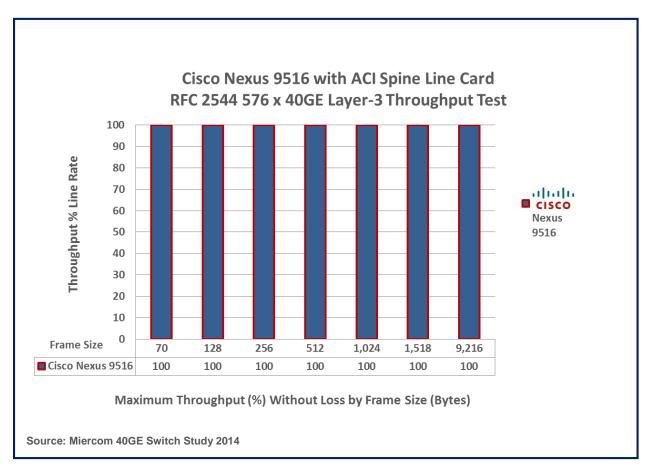
The Cisco Nexus 9516 with sixteen 36p 40G QSFP+ ACI spine line cards exhibits full line-rate forwarding performance with all 576 of its 40GE ports loaded. Test results shown are for 40GE port-pair testing, cross-fabric configuration. The switch was configured with 576 ports under maximum sustainable load without loss for Layer-3 (IP) unicast traffic for the particular frame size. Testing was conducted in accordance with RFC 2544.
