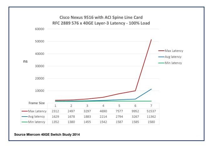
The Cisco Nexus 9516 exhibits consistent low latency for the full range of packet sizes tested across all 576 of its 40GE ports with 100 percent load on all ports. From the smallest packet size of 70-Bytes to the largest 9216-Bytes, the average latency ranges from 1.6 to 11.4 microseconds. Results are shown for 576 x 40GE full-mesh testing at 100 percent traffic load. Tests were conducted in accordance with RFC 2889.
