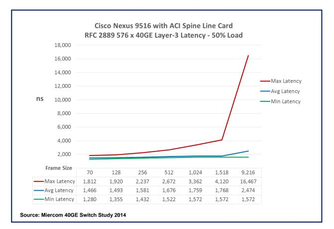
The Cisco Nexus 9516 exhibits consistent low latency for the full range of packet sizes tested across all 576 of its 40GE ports with 50 percent load on all ports. From the smallest packet size of 70-Bytes to the largest 9216-Bytes, the average latency ranges from 1.5 to 2.5 microseconds. Results are shown for 576 x 40GE full-mesh testing at 50 percent traffic load. Tests were conducted in accordance with RFC 2889.
