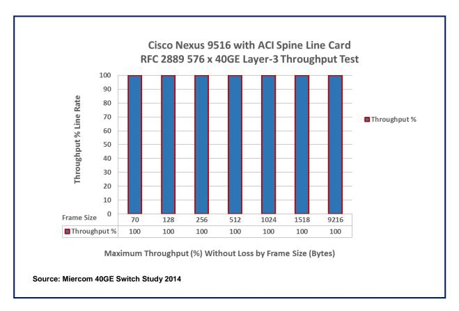
The Cisco Nexus 9516 exhibits full-line-rate traffic handling across 576 x 40GE ports loaded. These results are for testing of 40GE ports in a cross-fabric configuration, with full-mesh traffic loads. Tests subjected the switch to the maximum sustainable load that it could maintain without loss of Layer-3 unicast traffic for the specified frame size. Tests were conducted in accordance with RFC 2889.
