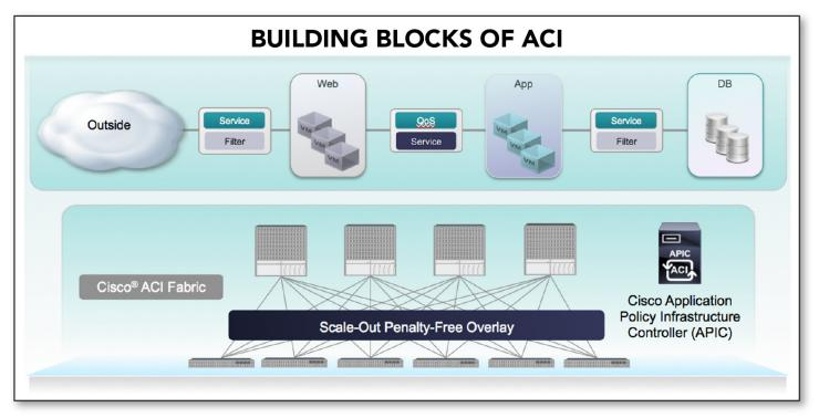
**Policy Model:** ACI's policy model creates a new way of describing connectivity via what Cisco calls the "Group-Based Policy" (GBP) concept. Cisco's policy model provides a generic way of describing how things connect. As an example, consider a typical three-tiered application deployed in a data center that may consist of a Web front-end tier, a middle-ware application tier, and a back-end database tier; this application may also need connectivity from the outside
