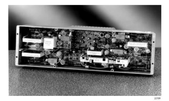
TYPE 1A SYSTEM AMPLIFIER III – 5-40/52-750 MHz
