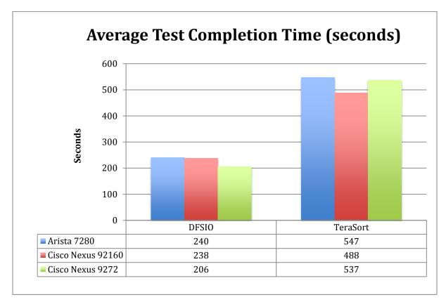
The test completion times across the platforms are comparable, even though some aspects of the switches – such as per-port buffer depth – are quite varied.
