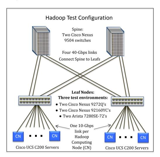
The test-bed data-center network featured two spine switches – Cisco Nexus 9504 modular switches with Cisco Nexus 9636Q Linecards. Each supported four 40-Gbps links, two to each "leaf" node, as shown above.
